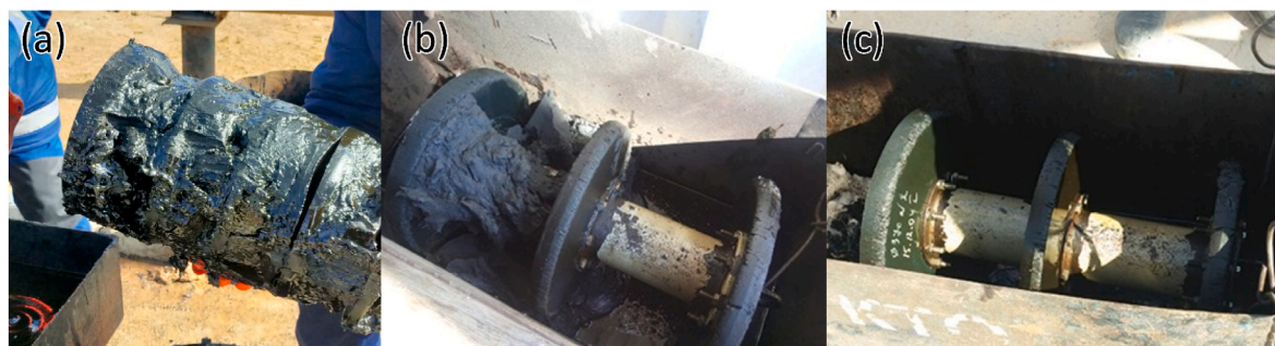
Fig. 9. The resulting pigs from untreated pipelines: (a) taken from the pipeline without PPD treatment, (b) received pig from the pipeline treated with 200 ppm EVA (Randep-5102), (c) received pig from the pipeline treated with 200 ppm gEVAST24C. The oil pipeline is 14.5 km long and 377 mm in diameter. Temperature gradient 60–25 °C.
