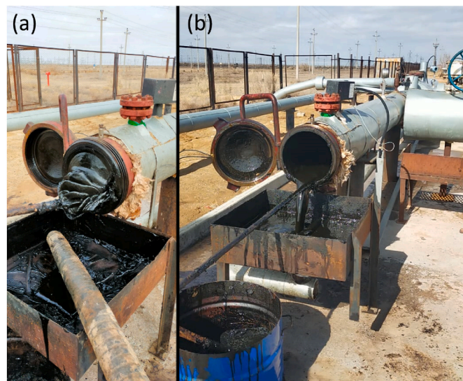
Fig. 8. Example of wax formation on a production line without PPD (a) and free-flowing oil treated with 200 ppm gEVAS24C (b).
